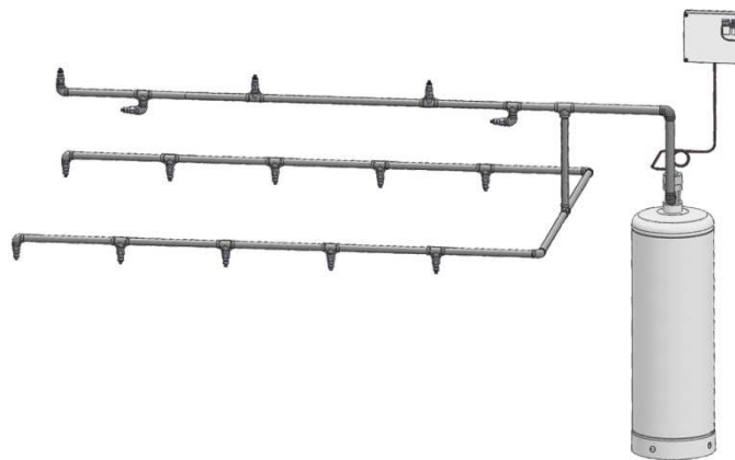
Figure 37: System example with three discharge lines
