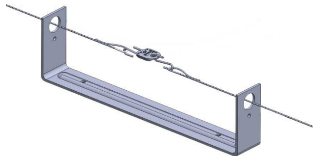
Figure 15: Detector mounting kit installation
