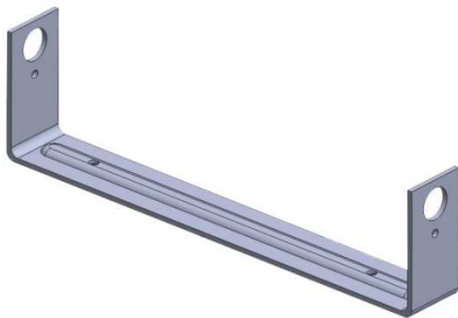
Figure 14: Detector mounting base
