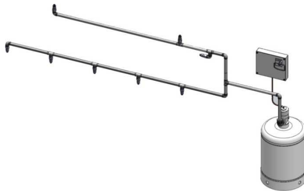
Figure 36: System example with two discharge lines
